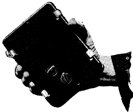
The smallest set: this Empiric Pocket Receiver is designed for headphone listening.
